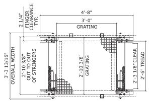
All standard crossover stairs (10", 19-1/2", 29", 38-1/2", 48" and 67" clearances) have 2'-6" wide stair treads and an overall width of 3' 3-13/16".
